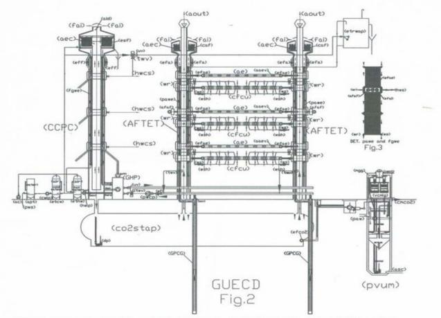
GUECD (GLOBAL URBAN ENVIRONMENTAL CONDITIONING AND DEPURATION) SCHEME FOR FUMES DEPURATION, CAPTURE CO2, AIR CONDITIONING, HEATING WATER CONSUME BY GAS HEAT PUMP AND LOW GEOTHERMAL ENTALPY. PLUS WATER DXIDATION WITH ALKALINIZATION, SLUDGE SEPARATION AND CO2 NEUTRALIZATION.
